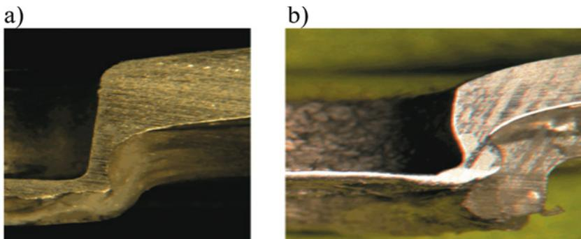
Fig. 27. Clinched joints of steel sheet with: a) – plastic; b) – carbon fibre composite
