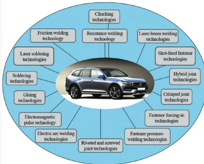
Fig. 2. Joining technologies used in the automotive industry
