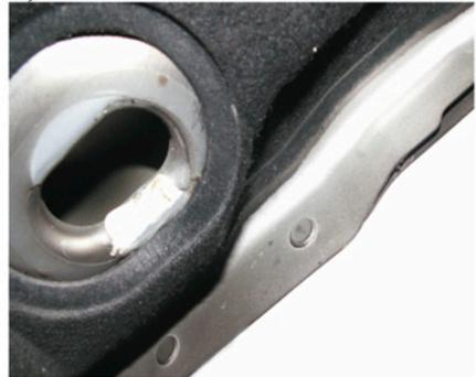
Fig. 23. Clinched joints in a Mercedes C-class: a) – fragment of the bonnet; b) – fragment of the boot lid
