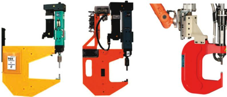
Fig. 11. Example designs of frames for industrial robots used for the assembly of motor vehicle bodies
