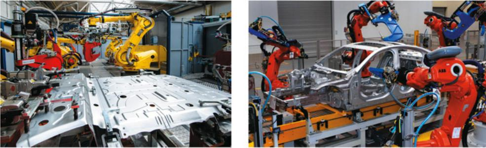
Fig. 9. Assembly workstations where the clinching technology is used
