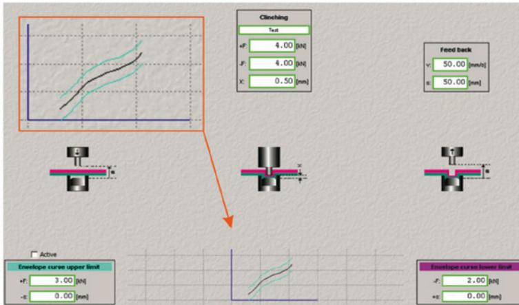
Fig. 13. Example window of a system to monitor the joint-forming force curve
