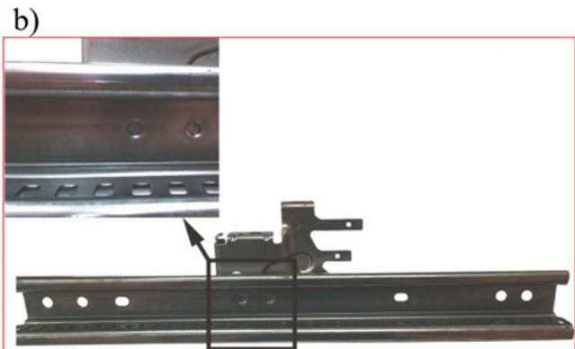
Fig. 19. Implementation of clinched joints in the construction of a vehicle seat: a) – seat frame; b) – seat sliding runner subassembly
