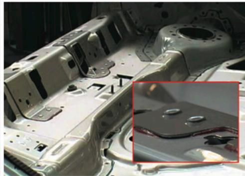
Fig. 28. Hybrid joint between sheet metal components of the Mercedes S-class body
